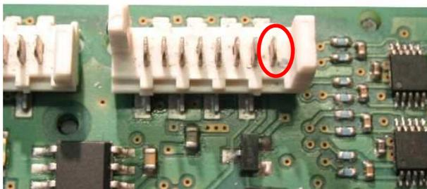
The connector is a MOLEX\_908140008, a suitable female connector would be a MOLEX - 90327-0308 like Farnell 673160.
