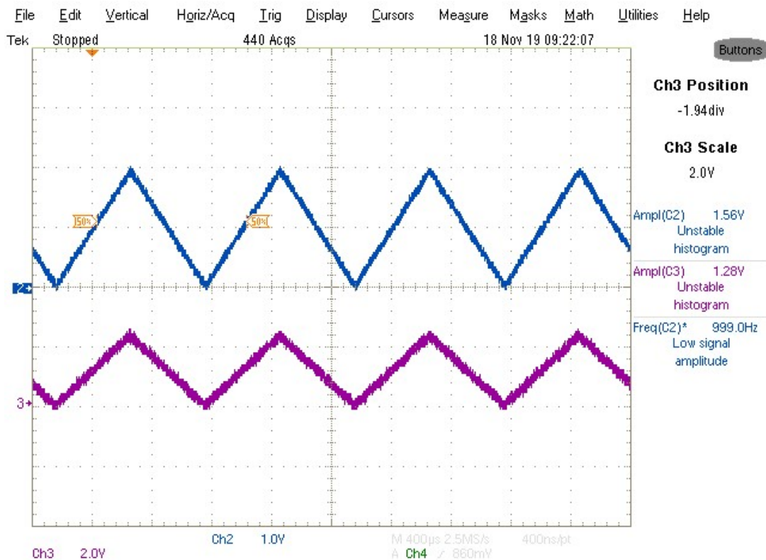
Picture 5: Blue: current monitor Purple: output current set (pin #10 of pin header #3)
