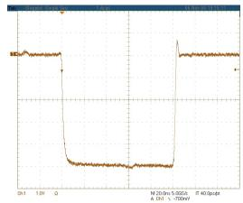
Figure: Current monitor output, scale: -2 A/Div
