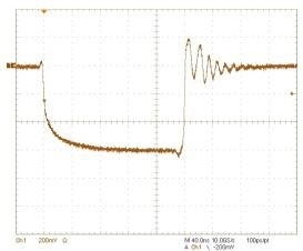
Figure: Current monitor output, scale: -80 A/Div
