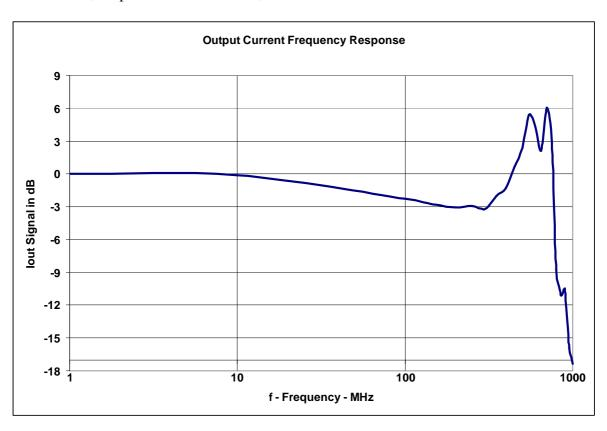
VCC = 15 V, output current = 125 mA, test load = short circuit.
