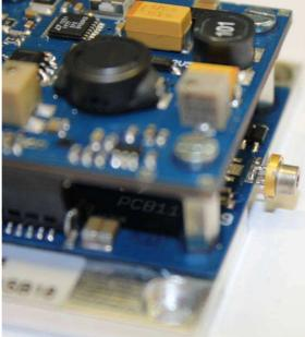
Laser diode connection: the rectangular pads on top (cathode) and bottom (anode). The dimensions of the rectangular pads are 1 mm x 5 mm. There is no optical feedback path. The unit is current controlled only.
