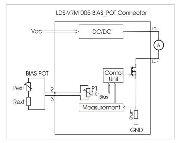
If the increase of Bias current is not necessary let pin 2 and 3 floating.
