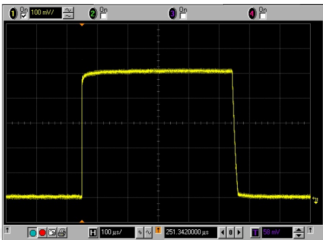
vertical 10 A/div, horizontal 100 \mu s/div pulse: 500 \mu s @ 50 A
